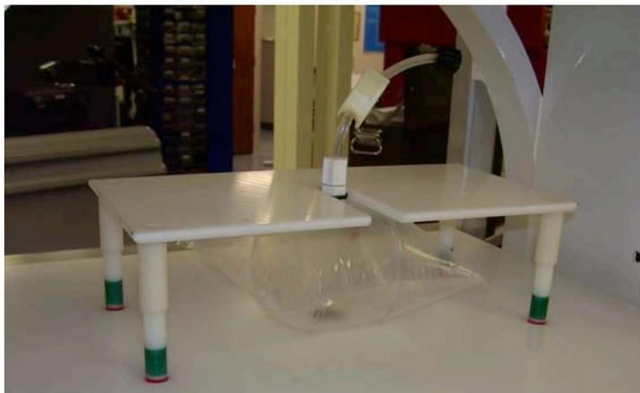
**Figure 5: Dose delivery bag filled with more than 1.1 liters of gas**
