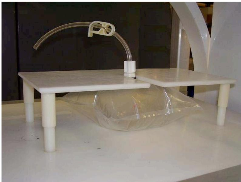
**Figure 2: Proper positioning of gas sample bag in Polarization Measurement Station**
