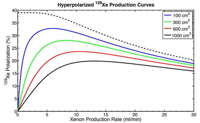
$^{129}\text{Xe}$  polarization as a function of production rate after installing the 3777 upgrade module.  $^{129}\text{Xe}$  polarization levels in the range of 20–25% are achievable using the standard 60W laser installed on 9800 systems. The dashed line shows the  $^{129}\text{Xe}$  polarization leaving the cell whereas the color-coded lines depict the collected xenon volume using an effective solid-state xenon relaxation time of one hour.
