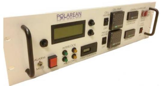
The new central control unit replaces the conventional temperature/interlock controller. In addition to providing the legacy functions, it regulates the rubidium pre-saturator function and provides enhanced monitoring and control of laser light transmission.
