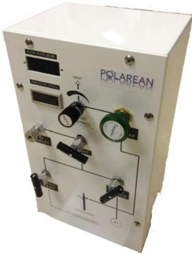
The upgraded outlet manifold thaw path is designed to improve user control and maximize  $^{129}\text{Xe}$  polarization retention during the thaw.
