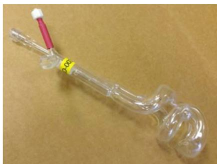
*An integral part of the polarized xenon collection system is the enhanced cryogenic trap – the cold finger, featuring an optimized geometry to enhance xenon freezing pattern and retention. This new design leads to a higher ultimate polarization of xenon through a longer solid-state relaxation time and an accelerated thaw into gas state.*
