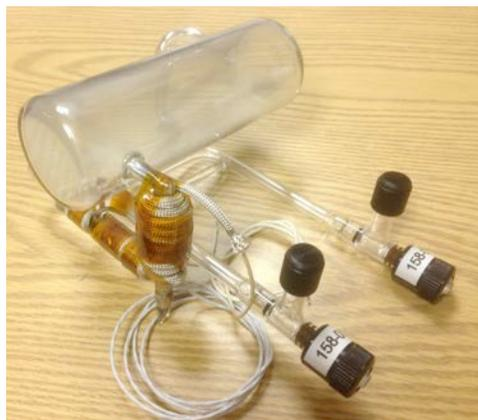
*The new optical cell design incorporates a pair of optical quality flat windows, a reinforced rubidium pre-saturator and a dedicated heater. The cell body is now largely free from rubidium and operates at a lower temperature than the rubidium pre-saturator in order to maximize spin exchange efficiency.*
