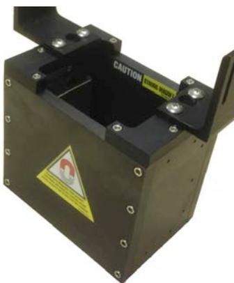
*The improved magnetic holding field minimizes polarization loss during xenon collection and recovery, and prolongs the polarization retention in solid-state xenon.*
